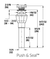
Ø1 Min to Ø1-1/2 Max. Deck Hole Openings
